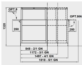
The large capacity of the well guarantees the display of a wide range of variations and tastes. Possibility to present from 9 up to 30 GN 1/6 h 200mm containers.
